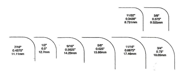
The smallest corner radius we can do is 11/32" due to the way the corners are tucked. Anything smaller would need to be square.
